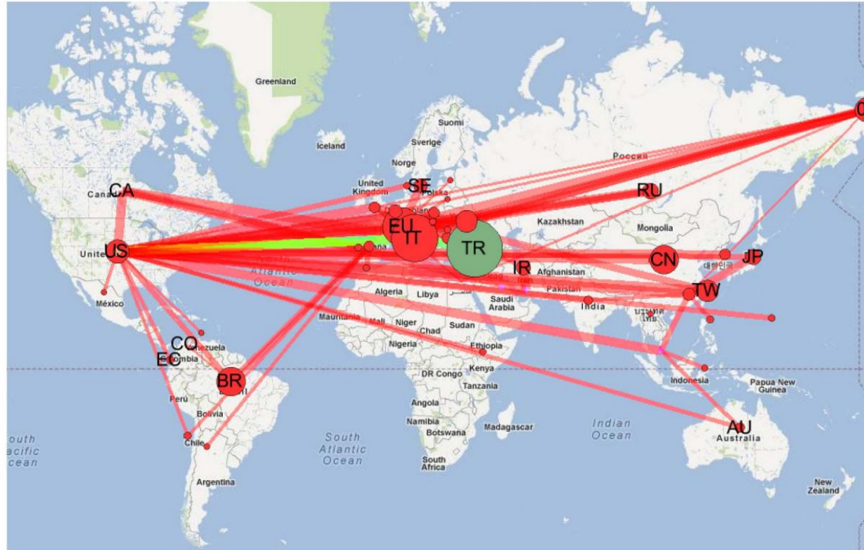
Fig. 5. Country-view of the BGP Hijacking event on 24-Dec-2004 around 9:24 GMT. Turkey gains most of the Internet traffic while most of the rest of the world lose traffic. The monitoring point is the orange colored node (AS-3549) located in US.
